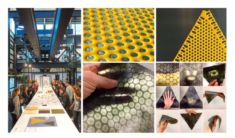
The recent "Biofabricate Summit" exhibit (<u>https://www.biofabricate.co</u>) at the New Lab NYC showcased leatherlike biomaterials based on silk protein with augmented edible and nutritional properties as well as thermochromic behavior. Developed by architect Laia Mogas and engineer Giusy Matzeu at the Living Materials Silklab, led by Dr. Fiorenzo Omenetto.
