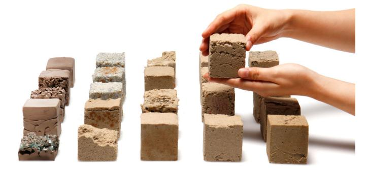
FINITE: A New Low-carbon, Bio-composite, Sustainable Replacement for Concrete https://urbannext.net/finite-low-carbon-bio-composite/
