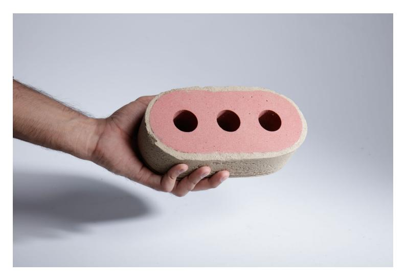
FINITE: A New Low-carbon, Bio-composite, Sustainable Replacement for Concrete https://urbannext.net/finite-low-carbon-bio-composite/
