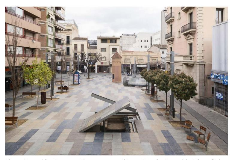
It has not been visited in 70 years. The new access will be created using two metal platforms flush with the pavement and covered to blend in with it, which can be lifted, pivoting on top of one another. The door emerges from underground attached to a single central piston. The entrance is only visible when open for a visit; it lies flush with the ground when the door is closed, disappearing without a trace.
