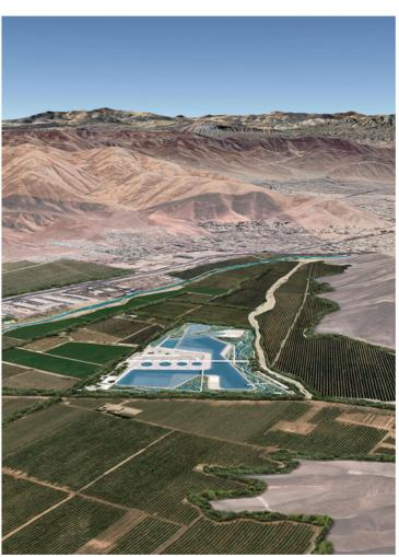
Due to the growing drought fueled by the climate crisis, in recent years a series of desalination plants have been built to supply water to the copper mining industry. Large underground aqueducts transport water from desalination plants (mostly powered by renewable energies) near the sea to mining areas up to 190 kilometers away and at an altitude of more than 4,000 msl.
