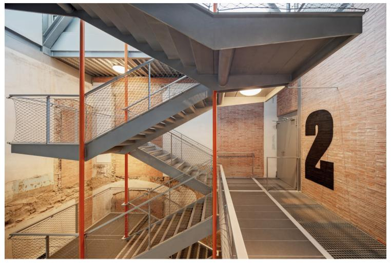
The project focuses on restoring the façade materials and recovering the original interior structure via an upper reinforcement with lightened concrete over the ceramic partitioned vaults supported by wooden beams resting on the existing iron columns.
