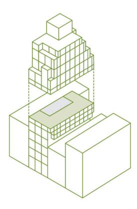
By proposing an access plaza on Franklin Place, we reduced the long dimension of the plate to 130 feet, but even that wasn't enough. The only effective remedy required openings on the party wall. Closing on an air right easement over 369 Broadway turned the north party wall, the longest wall of the building, into a third façade. Finally, a 10-foot cantilever came to compensate the area lost on Franklin Place's setback.
