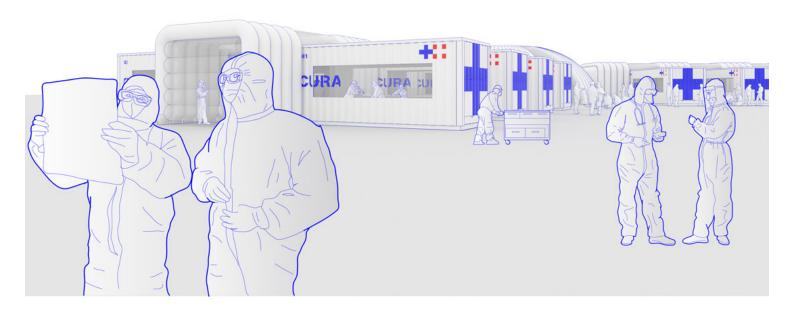
CURA is a compact intensive care pod for patients with respiratory infections, hosted in a 20-foot intermodal container with biocontainment (thanks to negative pressure). Each unit works autonomously and can be shipped anywhere. Individual pods are connected by an inflatable structure to create multiple modular configurations (from four beds to over 40), which can be
