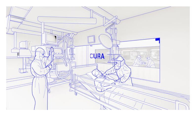
Each CURA pod would contain all the medical equipment needed for two COVID-19 intensive care patients – including ventilators and intravenous fluid stands. All units can be connected by an inflatable corridor. The first CURA pod is being built for testing at a hospital in Milan, Italy.
