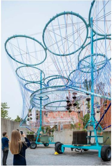
An assemblage of ecosystems, based on advanced environmental design, engineered to filter and purify 3,000 gallons of water, eliminating suspended particles and nitrates, balancing the pH, and increasing the level of dissolved oxygen.
