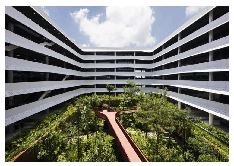
The building benefits from a rational floor plan and an exterior load bearing structure. This smartly maximises the floor layout and provides flexible interior space solutions.
