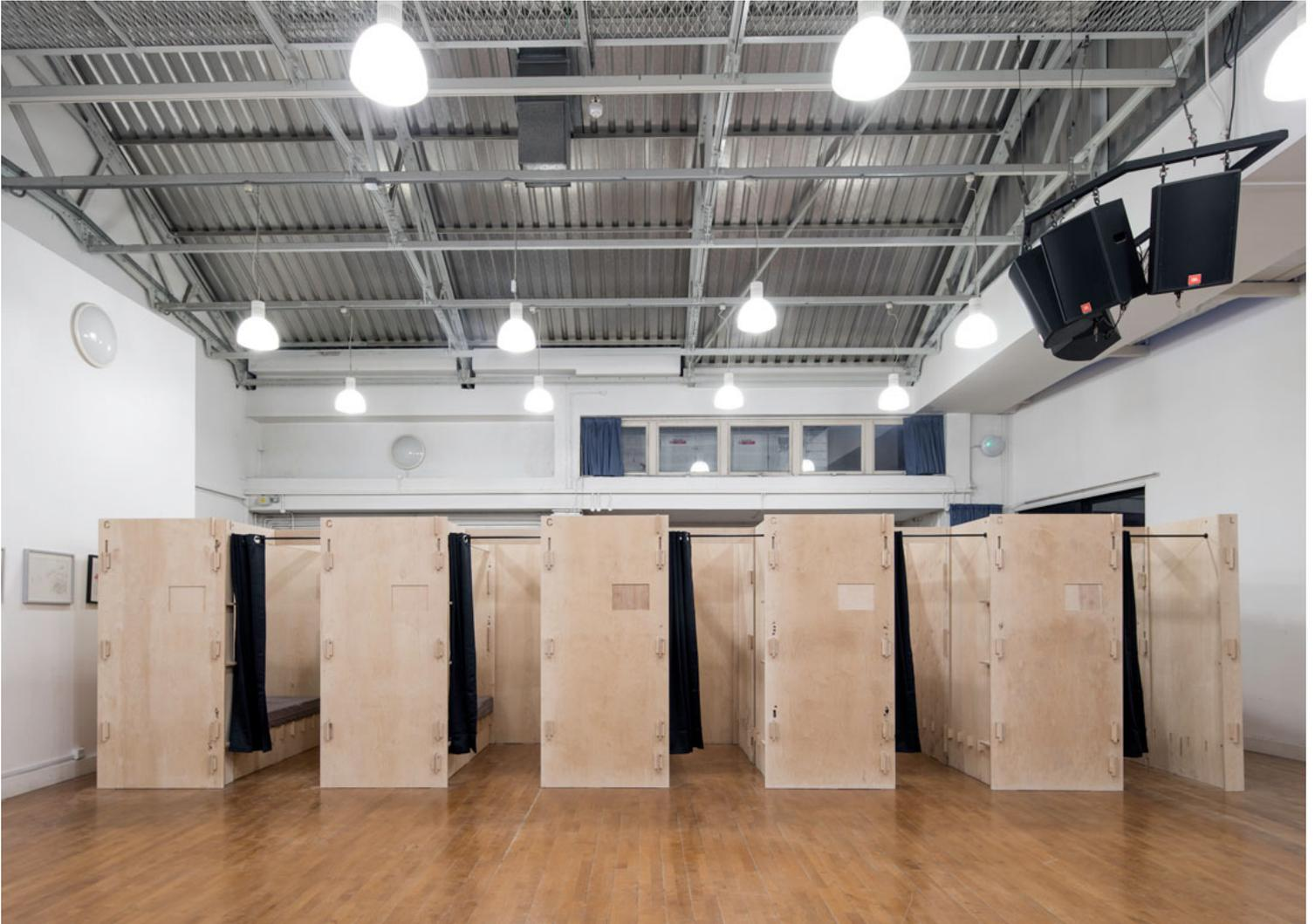
The pods stand 2.1 metres high, 2.1m in length and 1.9m wide, are made of 18mm thick, fireproof birch plywood and have privacy partitions with a raised platform for a mattress that acts as both a bed and a seat as well as storage space for personal belongings. Two of the side panels are shared with the adjacent pod, and a curtain on a rail can further close off the personal space at night-time.
