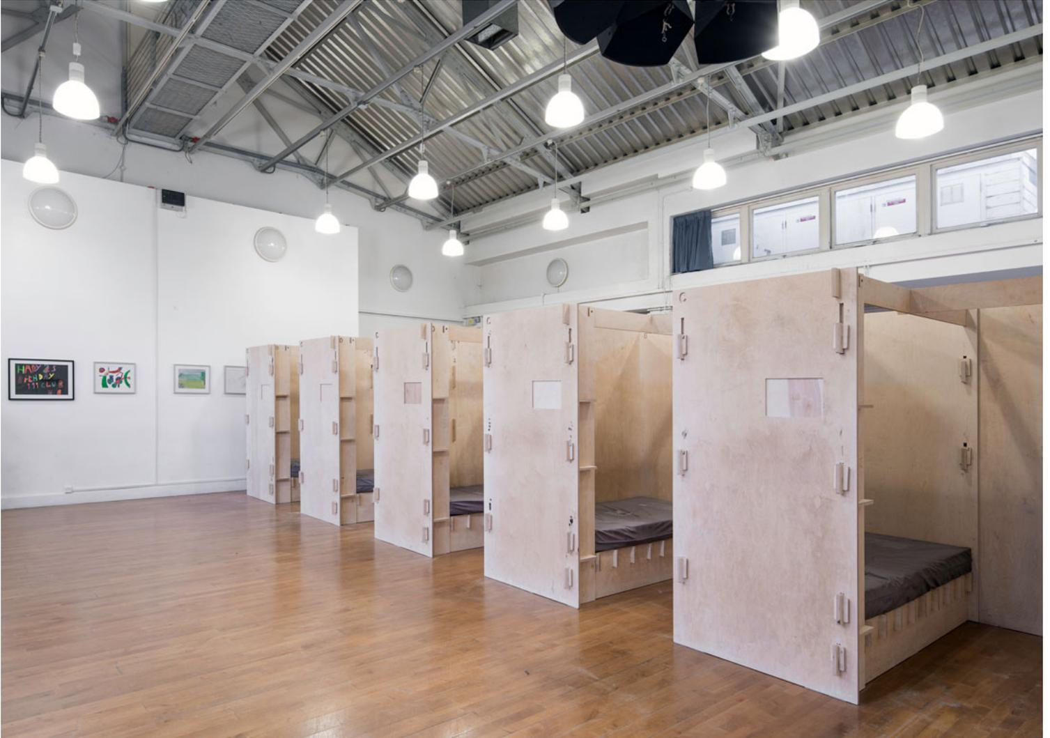
Following feedback from shelter management and guests, the initial model has been refined with its height reduced slightly to make it easier to install, and the raised mattress platform added to create the latest version.
