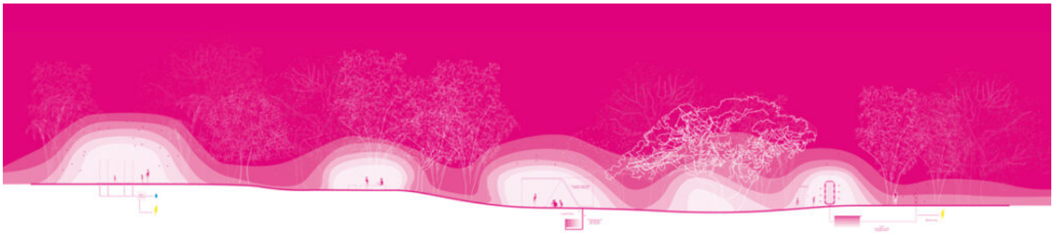
Fig. 1. Air temperature cross-section. Central Park, Taichung, Taiwan. In the heat represented in red, the white represents the colder areas in the park, cooled by shade, by convective air flows cooled by geothermal energy.
