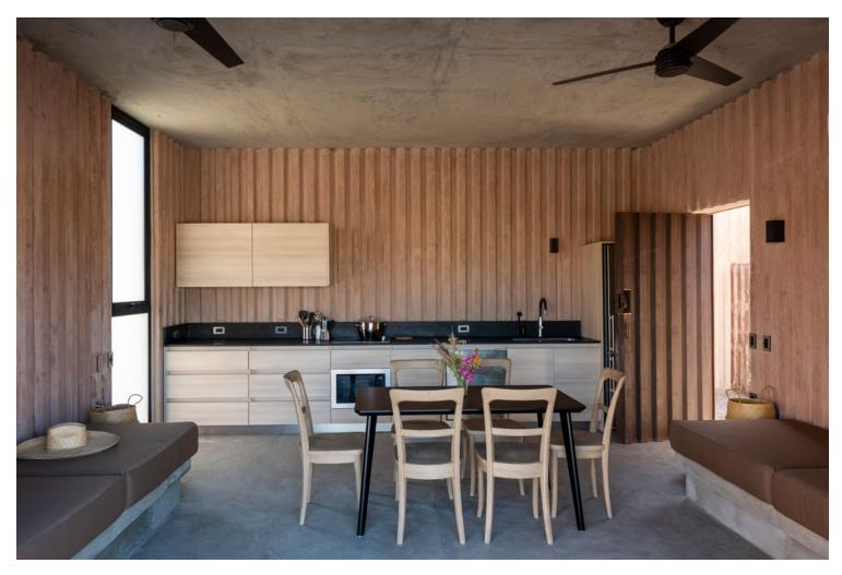
The unifying element of the house is concrete tinted a "sunset pink" color. The corrugated form serves as structure and finish at the same time. The channels provide geometry and visual rhythm to the interior and exterior spaces. At the same time, the walls offer insulation in a desert than can go from hot to cold in minutes. On the façades, the ribbed surface generates shade to reduce heat during the day. The concrete offers shelter in a seismic region that is exposed to oceanic change.
