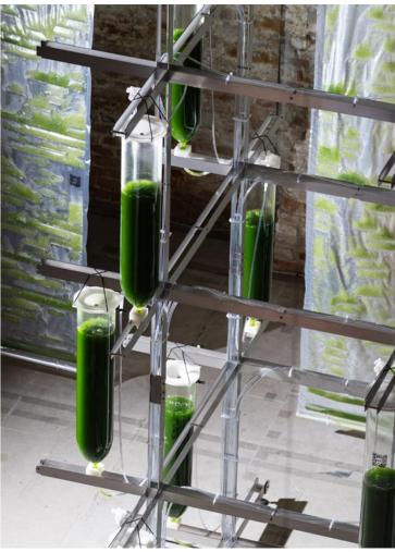
Each curtain is three meters high and one meter wide, and features 35 meters of digital welding, which forms a cavity capable of containing 7 liters of micro-algae cultures.
