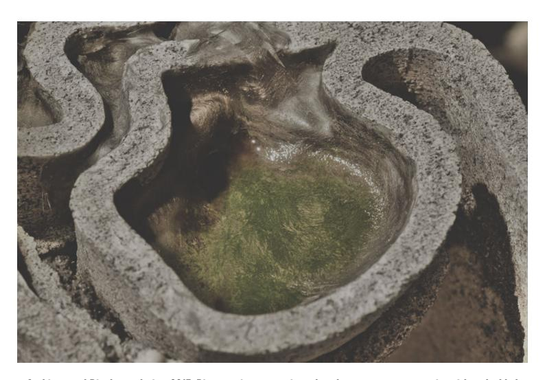
Architectural Biophotovoltaics, 2017. Bioreceptive magnesium phosphate concrete composite with embedded carbon fibre and algae in robotically extruded hydrogel to produce electric current.
