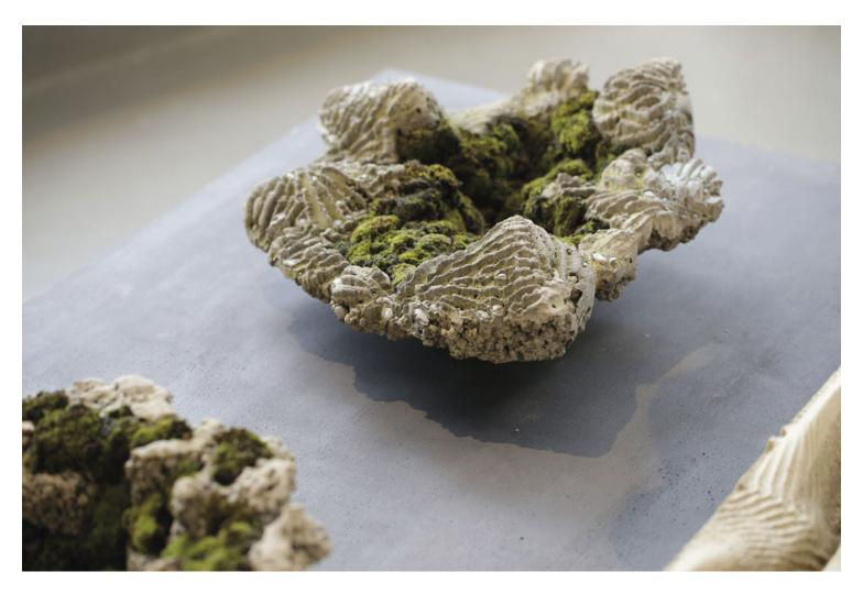
Bioreceptive lightweight concrete component with moss growth in exhibition at Super Materials, The Building Centre, London 2016 (components designed and built in 2015).
