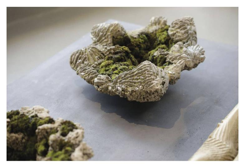
Bioreceptive lightweight concrete component with moss growth in exhibition at Super Materials, The Building Centre, London 2016 (components designed and built in 2015).
