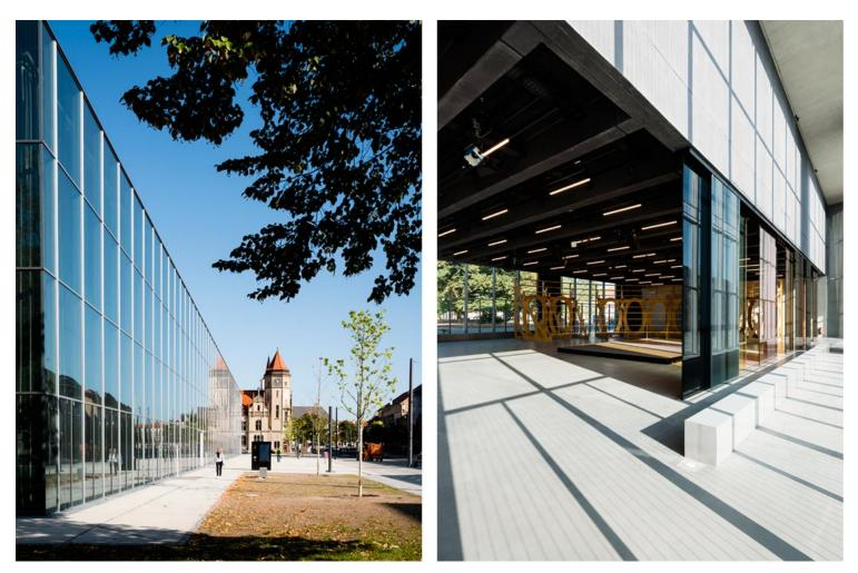
For the load-bearing structure, addenda architects took their cue from bridge building and pushed things to the limit. The cube thus rests only on two stairwell shafts, 50 meters apart, and there are no intervening supporting pillars. The two ends project about 18 meters over the stairwells. Beneath them, on the north side are office spaces and the delivery bay for art and, on the south side, event venues and education spaces.
