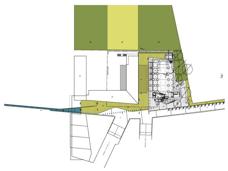
The new programmatic volumes inserted (as vertical accesses or technical equipment) have been located partially outside of the church with the aim of preserving the unity of the interior space of the nave. In addition, the new stairs and ramps provide a singular circular route across the building with amazing and diverse views.
