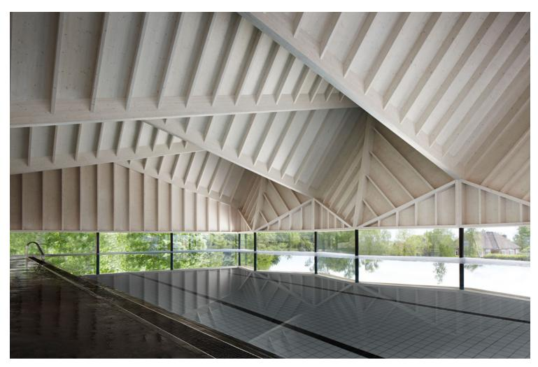
The new pool building sits discreetly at the rear of the site, facing directly onto the greenbelt land. Intended to be a contemporary expression of the local pitched roof vernacular, but executed with subtlety, the design of the new pool enclosure envisages a raised timber structure, articulated by three repeated folded roof segments.
