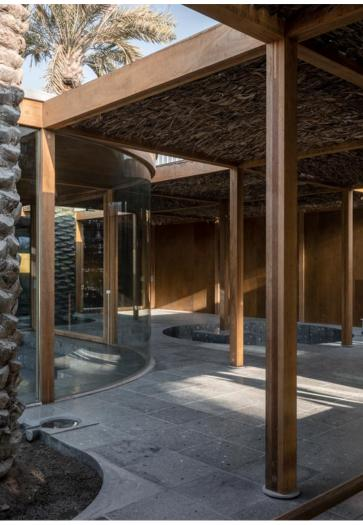
A tight grid of timber columns and beams is used on the site as both an organizing principle and a reference to the date palm plantations in the north of the island, irrigated by a complex network of water channels. The resulting building is a low single-story construction stretching the entire boundary of the site. Only the palm trees pierce through the horizontal ceiling to become the expression of the building.
