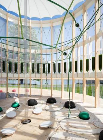
The filtering process is enhanced by the architectural morphology of the playground structure. The ETFE membrane – an evolution of the PhotoSynthetica urban curtain system presented in Dublin in 2018 by ecoLogicStudio – controls the microclimate inside AirBubble. The inverted conical roof membrane further stimulates the air recirculation and natural ventilation, which in turn keeps the play area clean.
