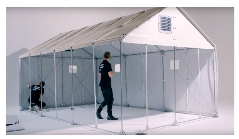
The Better Shelter resembles a very simple house. Its robust steel frame is clad with vertical, semi-hard walls, four windows, a high ceiling, and a door that can be locked. A solar-powered lamp provides light, and includes a USB port for charging electronic devices. The shelter is designed to last for three years, and is suitable for situations where local materials or construction workers are in short supply, with the additional value of preventing deforestation.
