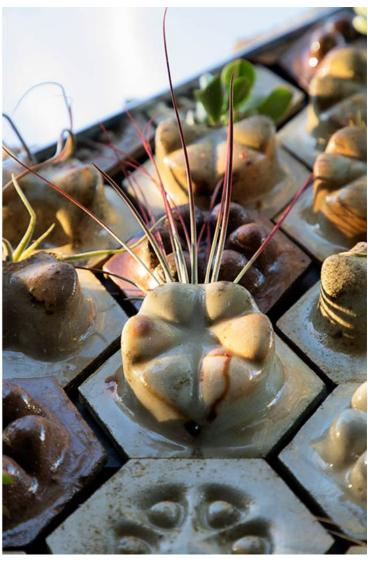
G-code is used to control each line of clay as it is 3D printed to create a loopy texture that looks like seeds scattered across the surface. While all ceramic tiles are printed from the same file, each tile is intentionally unique as a product of fabrication, during which the tiles wave back and forth, causing the printer to pull at the line of clay and creating longer and shorter loops toward the end of each tile, producing a distinct machine-made texture that is different every time.
