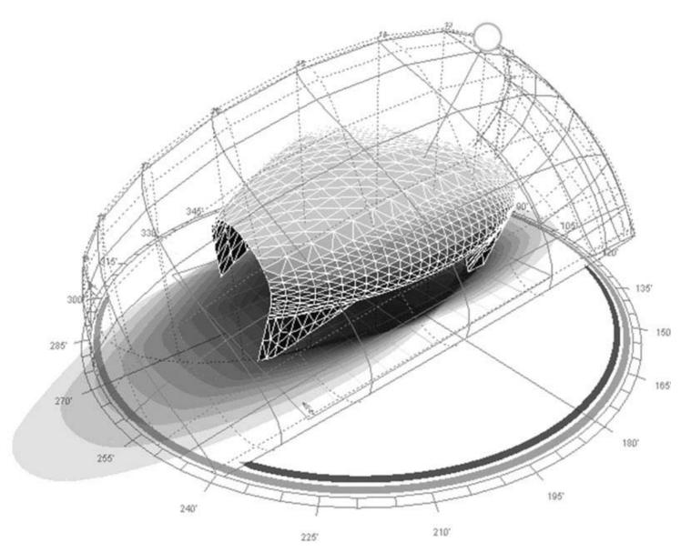
Our solar house also took on another challenge involving the inclusion of solar production in the building. We wanted to use a flexible photovoltaic material in order to produce a more naturally curved surface. We tried working with a new generation system based on technology like copper iridium gallium selenide (CIGS), but it wasn't available at the time, aside from the fact that its efficiency was only about 10%.
